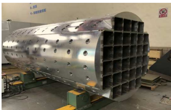
Stainless steel canister of NUHOMS ® being manufactured for the contract with CNNC/CGNP
